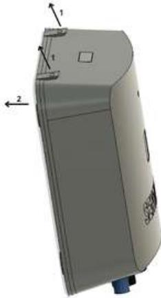
**2.** Attach the bracket to the wall using included self-tapping screws or adhesive tape. Be careful to retain the bracket orientation as the top and bottom clips on the bracket are different. Top clips are longer than bottom ones.
