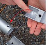
**Disassembling If you encounter difficulties** when disassembling the overlay tube, using two T-connectors can provide a better grip. This can be especially helpful in colder weather when it may be challenging to handle the 35mm tube effectively. Note once again that this is only recommended when disassembling the frame system.
