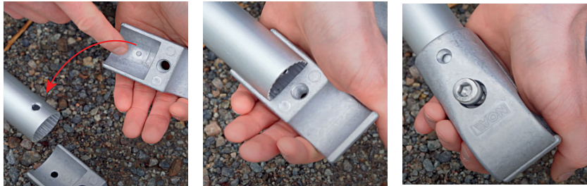
1. Position the spike to the hole on the tube 2. Hold the half with thread and spike 3. Put on the second half and fasten hex bolt
