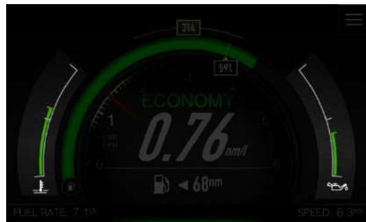
Following options are available for left or right gauge: fuel pressure, fuel level, oil level, electric drivetrain battery, electric drivetrain power, oil pressure, oil temperature, coolant pressure, engine temperature, engine trim, port trim tab and starboard trim tab.
