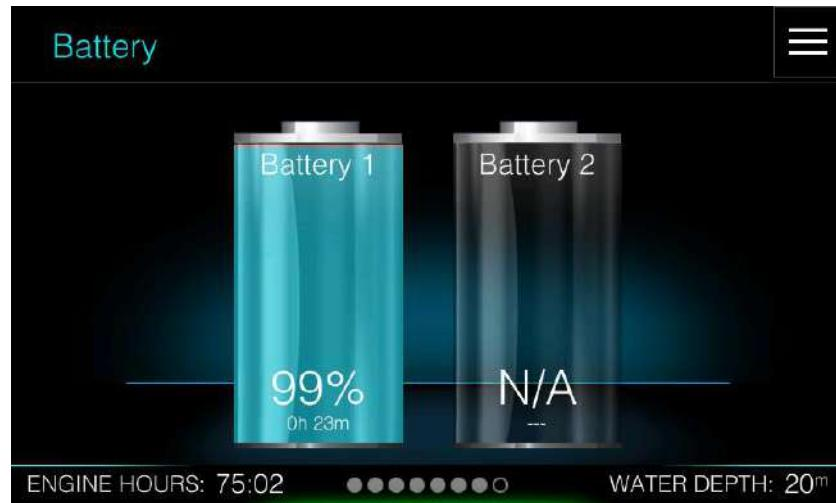
Battery information is available only if a SmartSHUNT or similar device is connected to the NMEA2000 network. SmartSHUNT is battery monitoring device, which constantly measures current, voltage and temperature of a battery and calculates state of charge and state of health of the battery.
