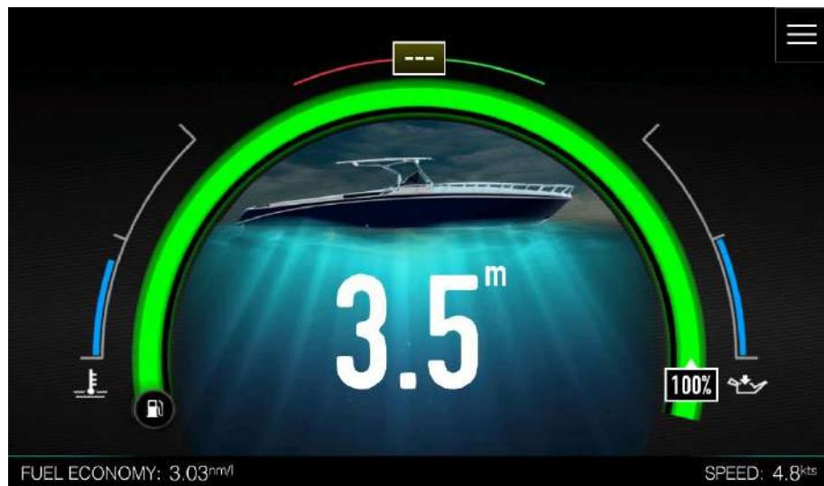
The dashboard screen is also used for IAssist function. The idea of dashboard screen is to show to the operator the right information at the right time. A smart logic is built-in device to choose right screen for a given situation. There is no need for the operator to search for requested parameter. A single most important value is shown on the centre of the screen.
